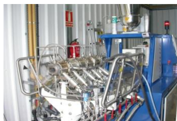
Twin-screw extruder at CIEMAT for biomass pretreatment
